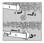
Open the rail stop flaps and pull the rack out completely. Now place it in high or low position, then slide it along the guide rails until the front wheels also go in. Now close the rail stop flaps. Follow the sequence of actions illustrated in figure "F'
